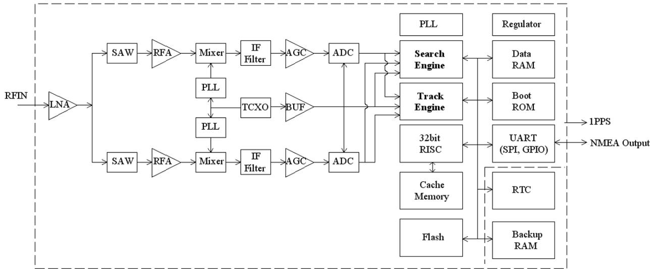
**Module block schematic**
